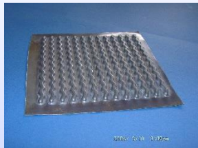
Wave structure for heat exchanger 1.4462, 0,15 mm
