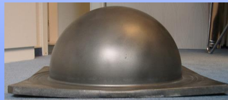
Hemisphere Submarine, \varnothing = 400mm, Ti6-4, s_0 = 20 mm
