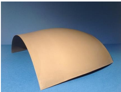
Fig.17: 120°-segment produced by HDD
