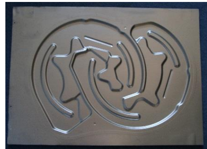
Fig.2: Heat shields Ti-6Al-4V
