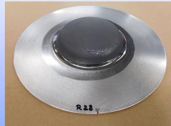
Hot stretch formed part R28 with Cassini bottom
